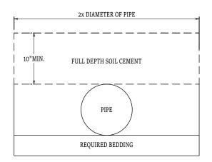
IF PREFERRED ISN'T POSSIBLE THEN AN ASPHALT OR CONCRETE PIPE SADDLE IS REQUIRED.
